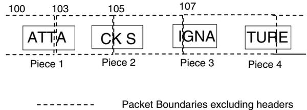
Figure 5: Example of Splitting each piece (packet boundaries are shown using dashed lines) into packets such that no complete piece is detected in a packet passing through the IPS
