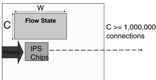
Figure 1: A model of a standard IPS integrated into a switch
