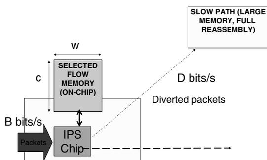
Figure 2: New model of an IPS with a fast path and a slow path
