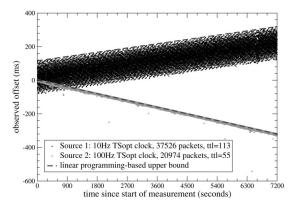
Fig. 1. TSopt clock offset-sets for two sources in  $BB_N$ . Trace recorded on an OC-48 link of a US Tier 1 ISP, 2004-04-28 19:30–21:30PDT. The source with the wide band has a 10 Hz TSopt clock, the source with the narrow band has a 100 Hz TSopt clock. A source with no clock skew would have a horizontal band.
