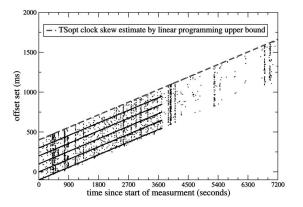
Fig. 6. TSopt clock skew estimate for a source in  $BB_s$ . Trace recorded on an OC-48 link of a US Tier 1 ISP, 2004-04-28 19:30–21:30PDT. TSopt clock skew estimate via linear programming: 175.2 ppm. Clock skew estimate via the Fourier transform: 175.6 ppm.
