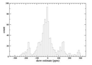
Fig. 2. Histogram of TSopt clock skew estimates for sources in BB<sub>N</sub>. Trace recorded on an OC-48 link of a US Tier 1 ISP, 2004-04-28 19:30–21:30PDT. Here, mp = 2000 packets, md = 50 minutes, and pv = 1 ppm.
